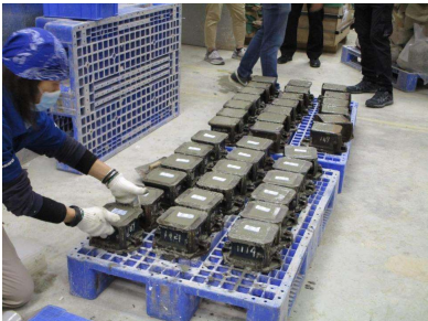
Casting specimens with concrete mix utilized for calibration process
