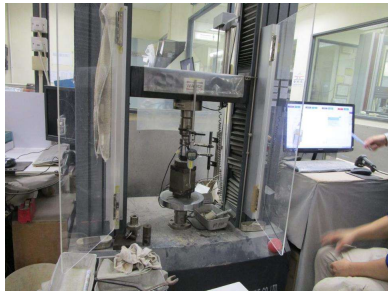
Determination of compressive strengths at pre-established times and for each curing temperature
