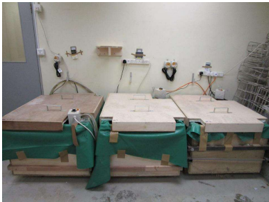
Curing at 3 different temperatures as required to extract maturity model parameters
